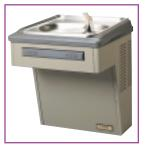
Unit complies with Americans With Disabilities Act when properly installed and is lead free. The dispenser uses bubbler-type pressure to produce 6 gal per hour. Compressor runs on 115v, 60-Hz, single-phase power. In accordance with CID A-A-2590.
