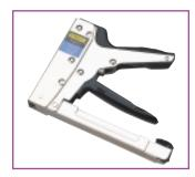
spring mechanism returns handle to starting position and feeds next staple to driving position, making it easier to operate with one hand. All surfaces are coated to prevent corrosion. Comfortable handgrip design. Tacker accepts 1/2"-wide flat crown staples. Sizes 4 (1/4"), 5(5/16"), 6(3/8") and 7(1/2" leg lengths). Tacker accommodates at least 84 staples. Use for posters, labels, tags and building paper.
