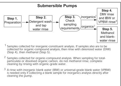
**Figure 3–5.** Cleaning procedures for submersible pumps.
