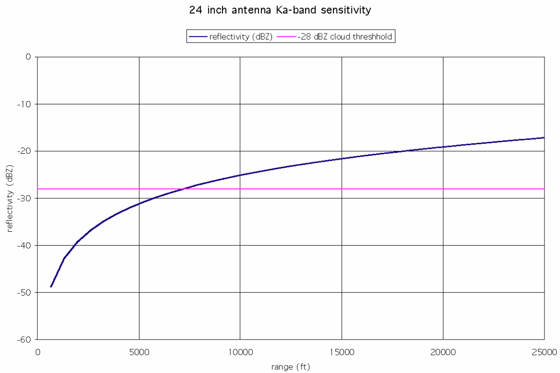
Figure 3.—Ka-band radar (with 24 inch antenna) minimum detectable reflectivity.
