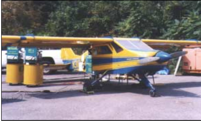
Figure 2.2 - WVU STOL Research Aircraft Containing the GTC-85-72 Gas Turbine Engine and View Looking Down its Exhaust Stack
