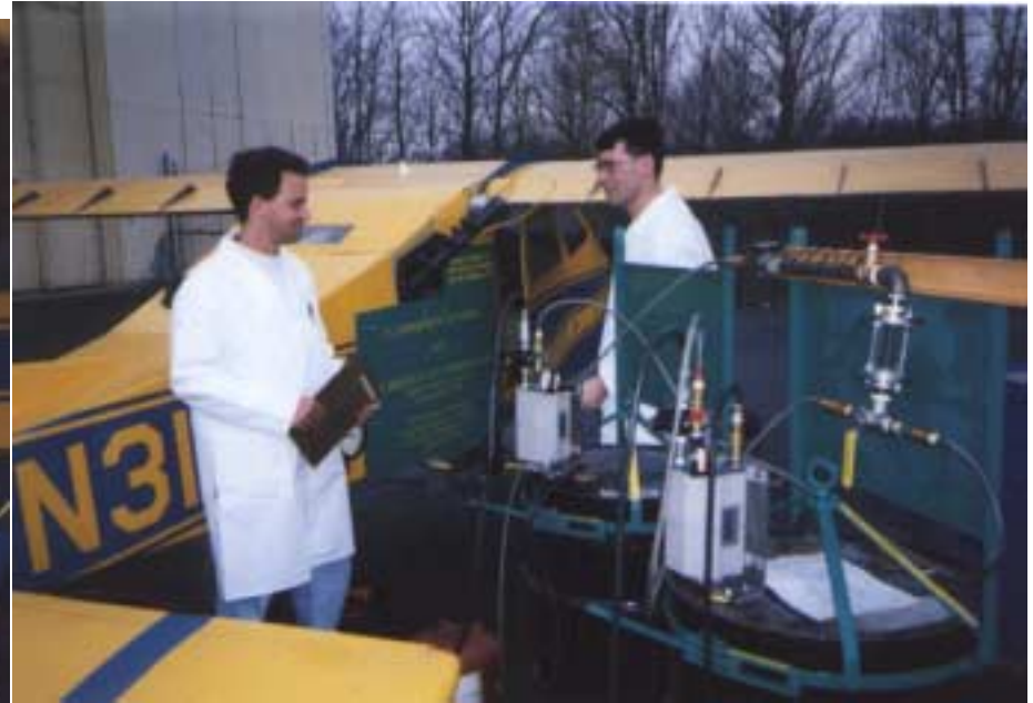
Figure 2.1 -Photographs of Instrumentation, Controls and Bleed Air Manifold Shown with Operator Protective Shield
