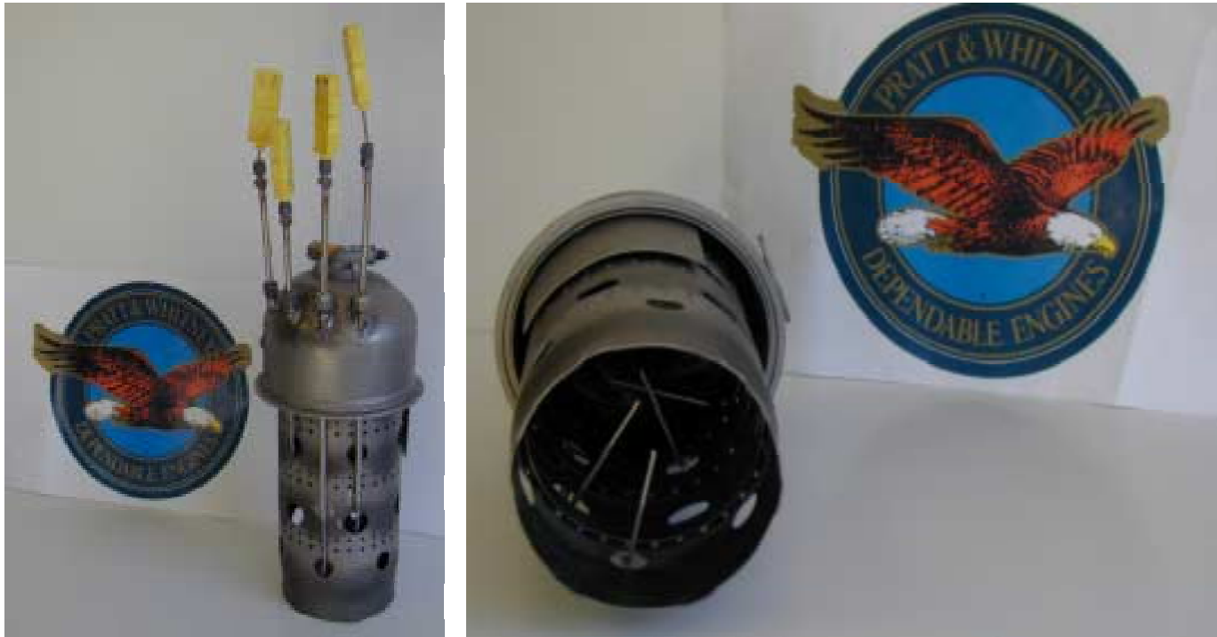
Figure 4.1 - Photographs of Thermocouple Equipped Combustor Can as Modified by WVU and Pratt and Whitney Canada
