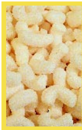
Biodegradable loosefill packing material is 95 percent starch and 5 percent synthetic polymer. (K7203-15)
