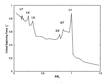
FIG. 10. Critical depinning force  $f_p^c$  versus vortex density for a triangular pinning array. Commensuration peaks can be seen at  $B/B_{\phi} = 1/1$ , 6/7, 2/3, 1/3, 1/4, and 2/7. Note that there is no peak at  $B/B_{\phi} = 1/2$ .
