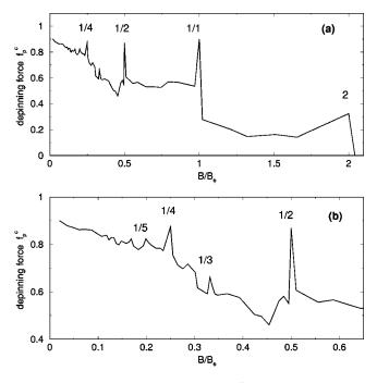
FIG. 1. (a) Critical depinning force  $f_p^c$  versus vortex density  $B/B_{\phi}$  for  $0 < B/B_{\phi} < 2.1$  with a square pinning array. Peaks can be seen in  $f_p^c$  at  $B/B_{\phi} = 1/4$ , 1/2, 1/1, and 2/1. (b) Critical depinning force for the system in (a) for  $0 < B/B_{\phi} < 0.6$  showing narrowed view of the peaks in  $f_p^c$  for  $B/B_{\phi} = 1/5$ , 1/4, 1/3, and 1/2. Smaller peaks can also be seen at  $B/B_{\phi} = 2/7$ , 1/6, and 1/8.
