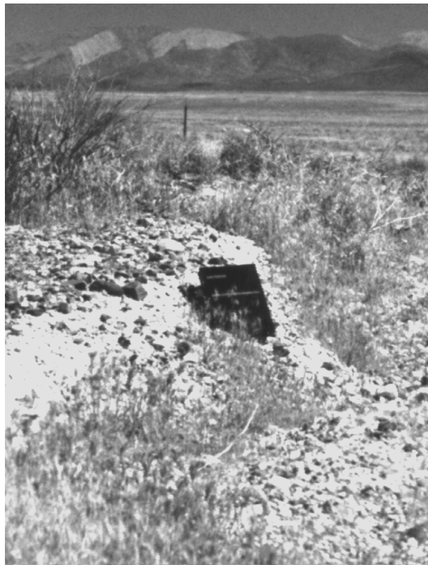
Figure 15. Reactivation of movement along an existing fault near the test area (Kinibito), showing offset of desert pavement (just to the top left of the field notebook shown for scale). Along this fault, which was only prominent near the test area, the soil was disturbed, being inflated or “fluffed” as a result of rapid vertical acceleration and slap-down not characteristic of natural tectonic movement.
