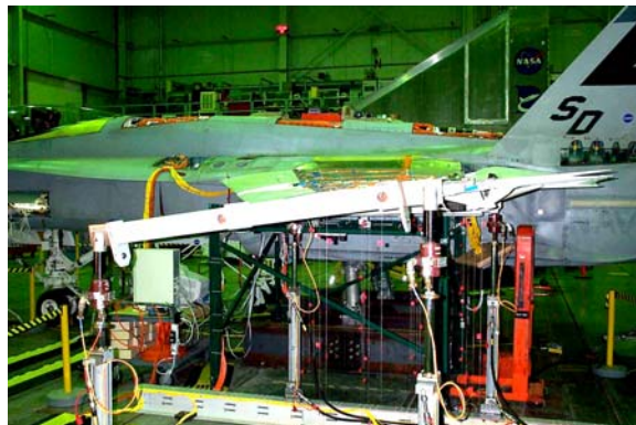
Figure 1. AAW Left Wing Under Negative Torque Load
