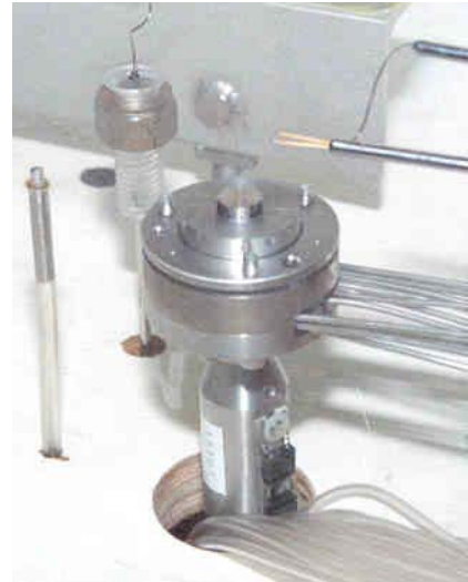
Figure 1. Photograph of skin friction sensor and reference instrumentation in Washington University Low-Speed Wind Tunnel
