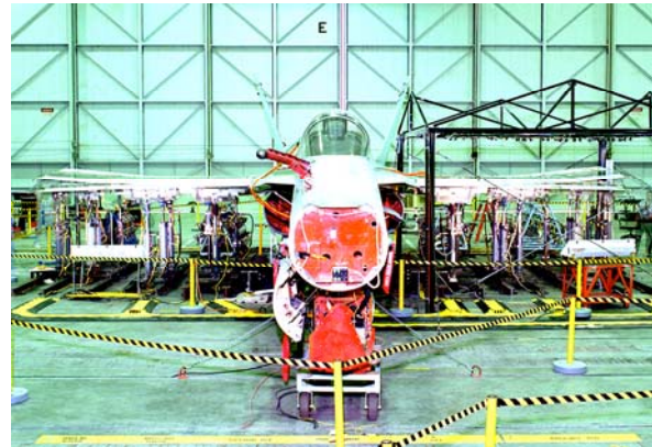
Figure 1. AAW Under 0% and 100% Load (Composite Photo)
