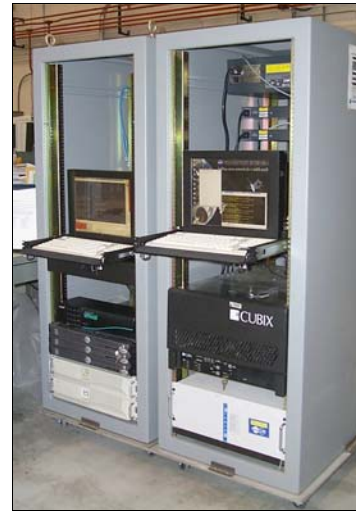
Fig. 1. Front view of prototype second generation remote site node containing multiple servers, network firewall and switches, and uninterruptible power supplies.
