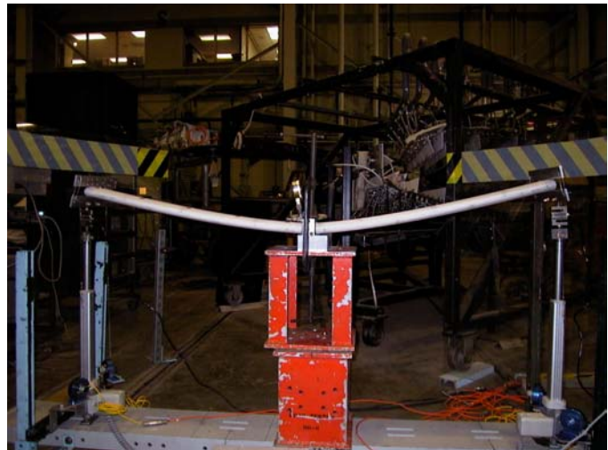
Figure 1 - Static structural testing of the inflatable wing
