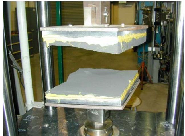
2" thick Neoprene load pad failed during Ultimate Strength Testing using a Material Test Stand (MTS) machine
