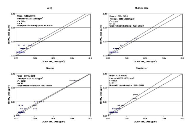
**Figure 1.** Comparison of PM10 lead concentrations from an Andersen high-volume  $PM_{10}$  on QMA quartz-fiber filters analyzed by AAS and a Sierra 241 dichotomous  $PM_{10}/PM_{2.5}$  sampler with Teflonmembrane filters analyzed by XRF (Watson et al., 1999a) at the four sites during the third year of the Robbins Particulate Study in South Chicago between 10/01/97 and 09/26/98 (Watson et al., 2000).
