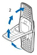
3 Turn the phone to a horizontal position and hold is as shown.
