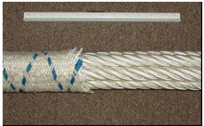
Figure 4.- Mooring rope constructed of seven subropes and encapsulated in a braided outer cover. (Manufactured by Whithill Manufacturing Company)
