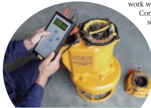
BJM technician performs a pump test
