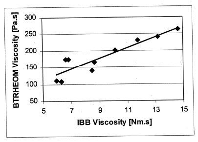
Figure 2: Comparison between the two rheometers: IBB and BTRHEOM
