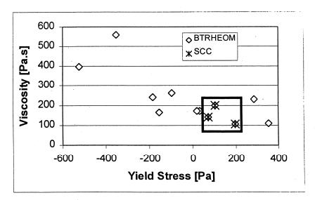
Figure 4: Viscosity vs. Yield stress calculated according to Bingham equation and the workability box
