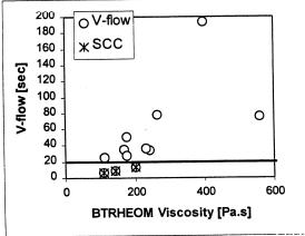
Figure 3: U-flow and V-flow time compared with viscosity measured with the BTRHEOM.
