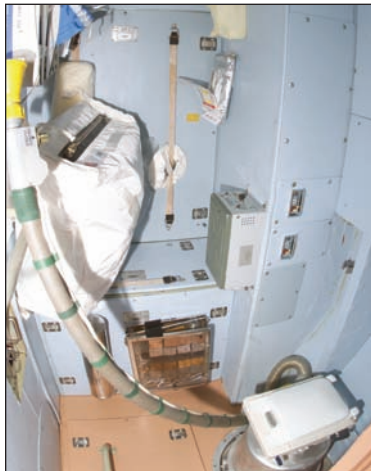
Using the bathroom without gravity is a different experience. The toilet aboard the space station doesn't require flushing because it has fans that suck air and urine through the funnel and hose into the wastewater tank.
