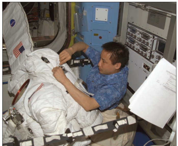
Astronaut Edward T. Lu, Expedition 7 NASA ISS science officer and flight engineer, performs routine maintenance on an extravehicular mobility unit space suit in the Quest airlock on the International Space Station.
