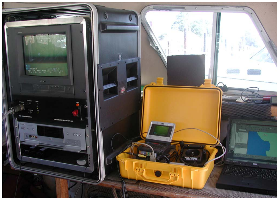
Figure 1.5 Data acquisition for the camera SLED included a DVD recorder, monitor, and text overlay unit housed in ocean-going black case (left). Video from the SEAVIEWER system was recorded on a Digital-8 tape deck (in yellow waterproof box, center) after the. GPS data was burned onto the video image and written to the audio track. A PC Laptop (right) displayed track lines for navigation, recorded incoming GPS position data, and output display topside for captain's navigation.
