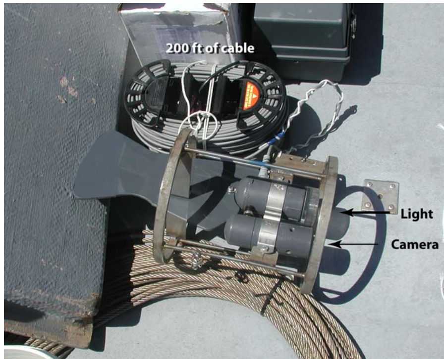
Figure 1.4 Photograph of the SEAVIEWER camera system rigged to collect towed video.
