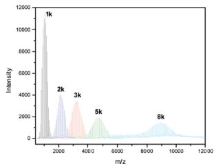
Figure 4. MALDI-TOF MS of a series of PEGDMs.
