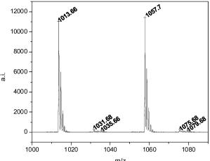
Figure 3. MALDI-TOF MS of 1k PEGDM, (a) full spectra and (b) expansion showing one main set of peaks 44 u apart due to Na+ cationized PEGDM and two minor sets of peaks of PEGDM cationized by K<sup>+</sup> and H<sup>+</sup>, respectively.
