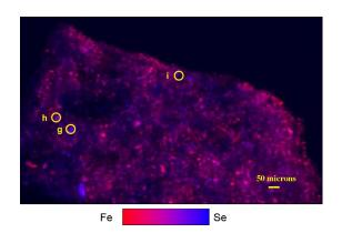
FIG. 4. (Color) Bi-color micro-SXRF map of middle waste shale sample 2. Letters on circles indicate points of interest.
