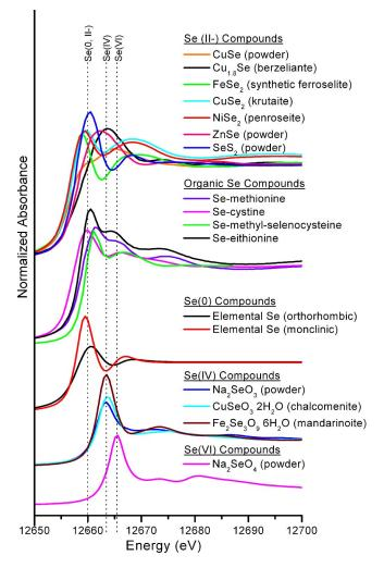
FIG. 2. (Color) Selenium XANES spectra for reference standards.
