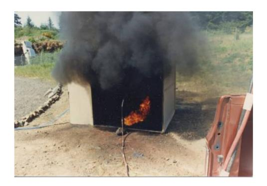
Fire spreading to resin on back wall of booth...resin spray continues but does not burn.
