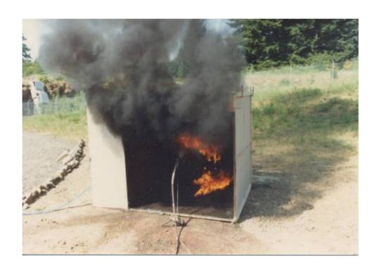
Resin burning on floor and back of booth, but resin spray is not burning.
