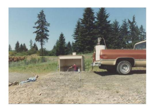
Start of resin spray. Spray will continue to allow accumulation of resin on floor and back wall. Duct in rear allows air flow.
