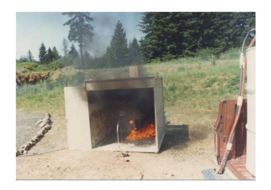
Resin on booth floor burning...resin spray does not burn.
