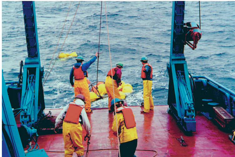
Figure 5. Mooring deployment. A , Instrument is a current meter with an attached transmissometer. B , Yellow spheres are subsurface floats.
