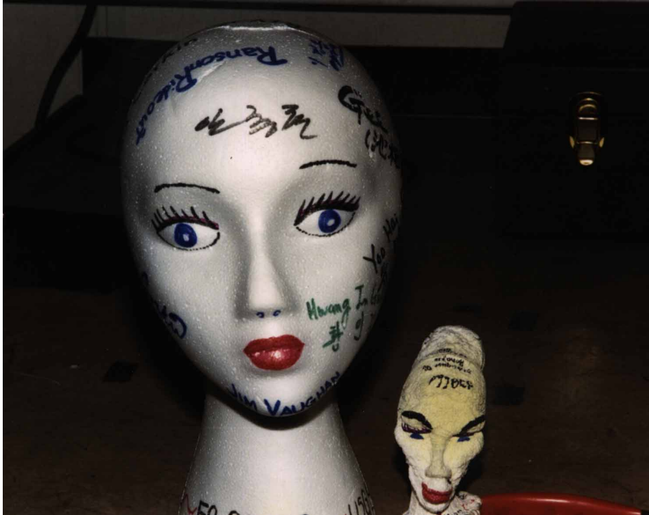
Figure 3. Two styrofoam heads. Head on right shows effect of pressure at 2,000-m (6,560 ft) water depth.
