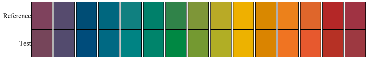
Figure 10: Simulated color appearance of 15 reflective samples when illuminated by the reference source (top row) and by test source B (bottom row).
