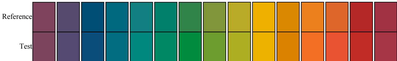
Figure 6: Simulated color appearance of 15 reflective samples when illuminated by the reference source (top rows) and by the test source (bottom rows).
