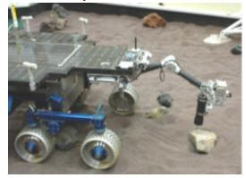
**FIGURE 15:** The USDC is shown drilling while mounted on the robotic arm of the FIDO Rover
