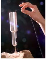
FIGURE 1: A photographic view of the USDC held from its cable while coring sandstone. The minimal need for axial force is easily seen.
