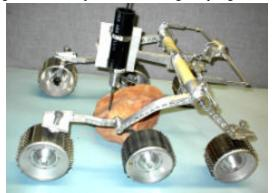
**FIGURE 14:** The USDC mounted on the Sojourner Rover platform is shown to drill sandstone.
