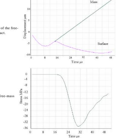
**FIGURE 8:** The displacement as a function of time of the freemass and the top surface of the drill stem after impact.
