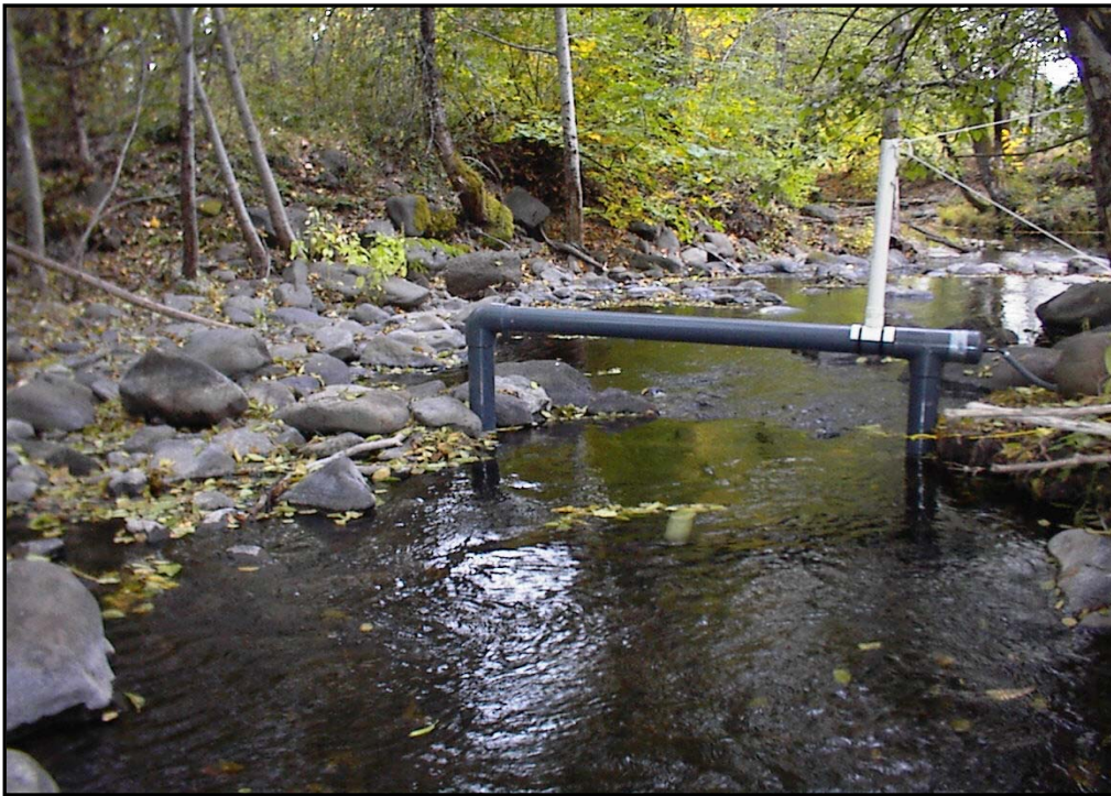
Figure 2. The pass-through antenna at low flow in Rattlesnake Creek.
