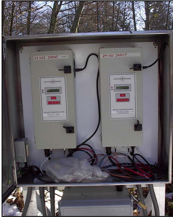
Figure 3. Transceivers and housing at Rattlesnake Creek.
