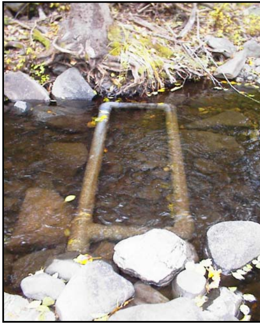
Figure 1. The pass-by antenna at low flow in Rattlesnake Creek.
