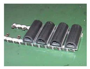
Figure -12 Crawler which D pattern midair rubber was used
