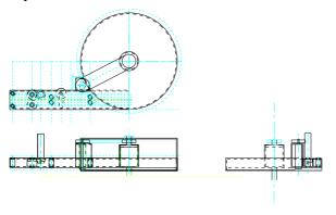
Figure -14 Wire wind device
