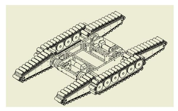
Figure -7 The internal structure of rescue robot
