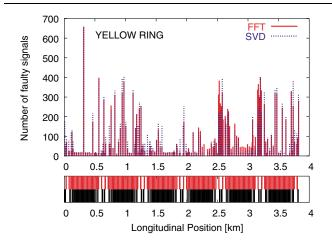
FIG. 12. (Color) Comparison of the FFT and SVD techniques for 678 files from the yellow ring showing a good agreement. The number of times a BPM provides a faulty signal is plotted versus its location.
