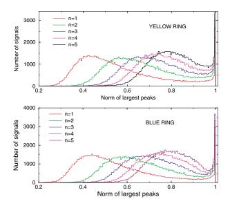
FIG. 10. (Color) Histograms of the norm of n largest peak values in each mode in the horizontal plane. Gaussian-like distributions represent coherent signal from good BPMs and peaks at 1 represent faulty BPMs.
