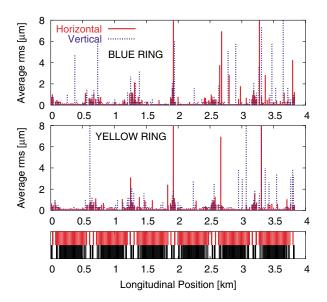
FIG. 14. (Color) Average rms observable versus longitudinal position of the BPM for run 2004.
