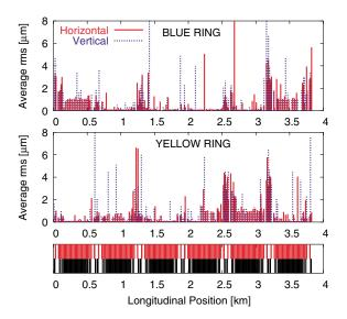
FIG. 8. (Color) Average rms observable versus longitudinal position of the BPM.
