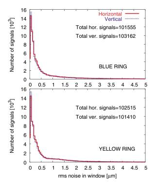
FIG. 6. (Color) Histograms of the rms observable for the two rings and the two planes. The total number of signals used in the histograms are shown.
