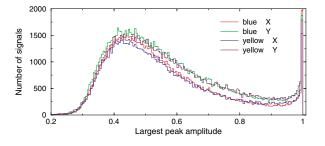
FIG. 9. (Color) Histogram of the largest peak amplitudes of all spatial modes for both planes in both rings. The Gaussian-like distributions represent a coherent signal from good BPMs and peaks at 1 represent faulty BPMs.
