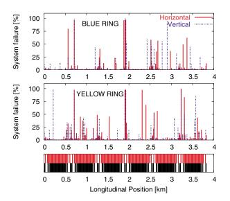
FIG. 4. (Color) Percentage of occurrences of system failure per BPM versus longitudinal location. A representation of the lattice (dipoles in black and quadrupoles in red) is shown in the bottom graph.
