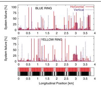
FIG. 13. (Color) Percentage of occurrences of system failure per BPM versus longitudinal location for run 2004. A representation of the lattice (dipoles in black and quadrupoles in red) is shown in the bottom graph.
