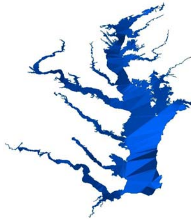
Figure 3-4: an exaggerated 3D view of the MHHW sea level surface within the Chesapeake Bay area.
