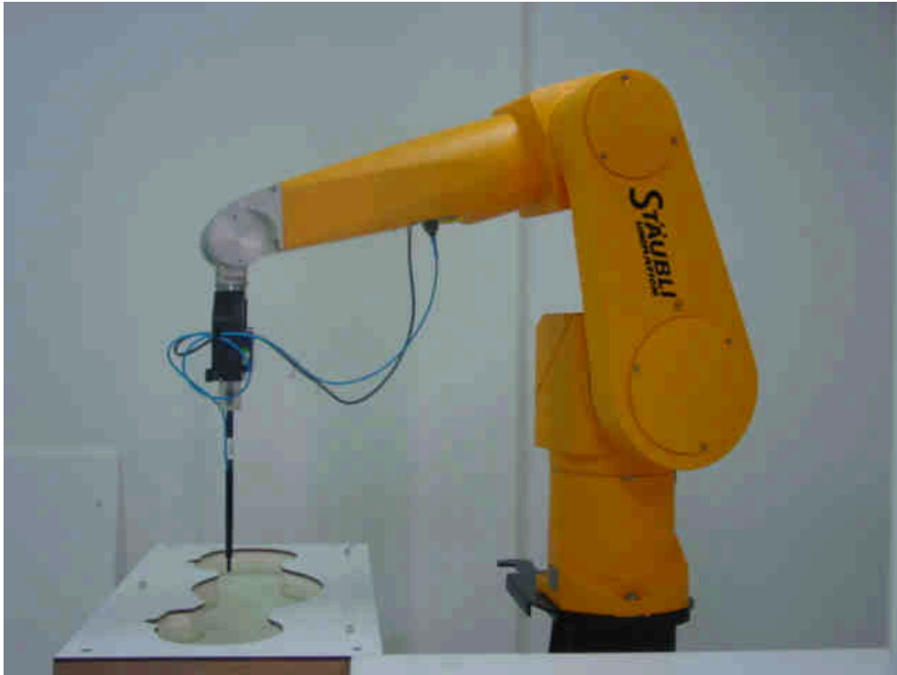
Picture B1: Specific Absorption Rate Test Layout
