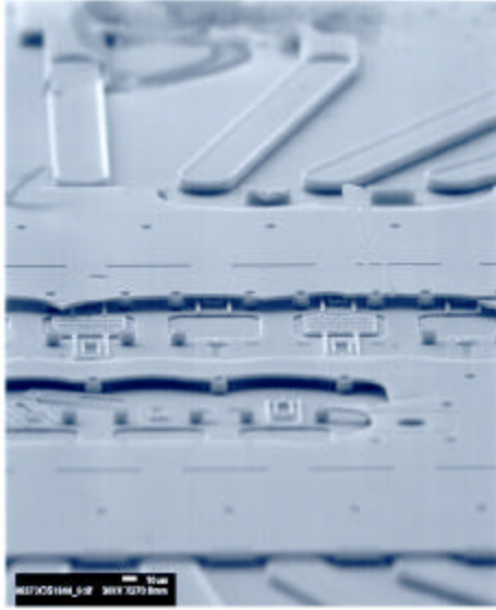
Figure 2. Electrostatic ejectors designed and fabricated using SUMMiT™ technology. Precise drop volume control without any satellite drop formation was achieved.
