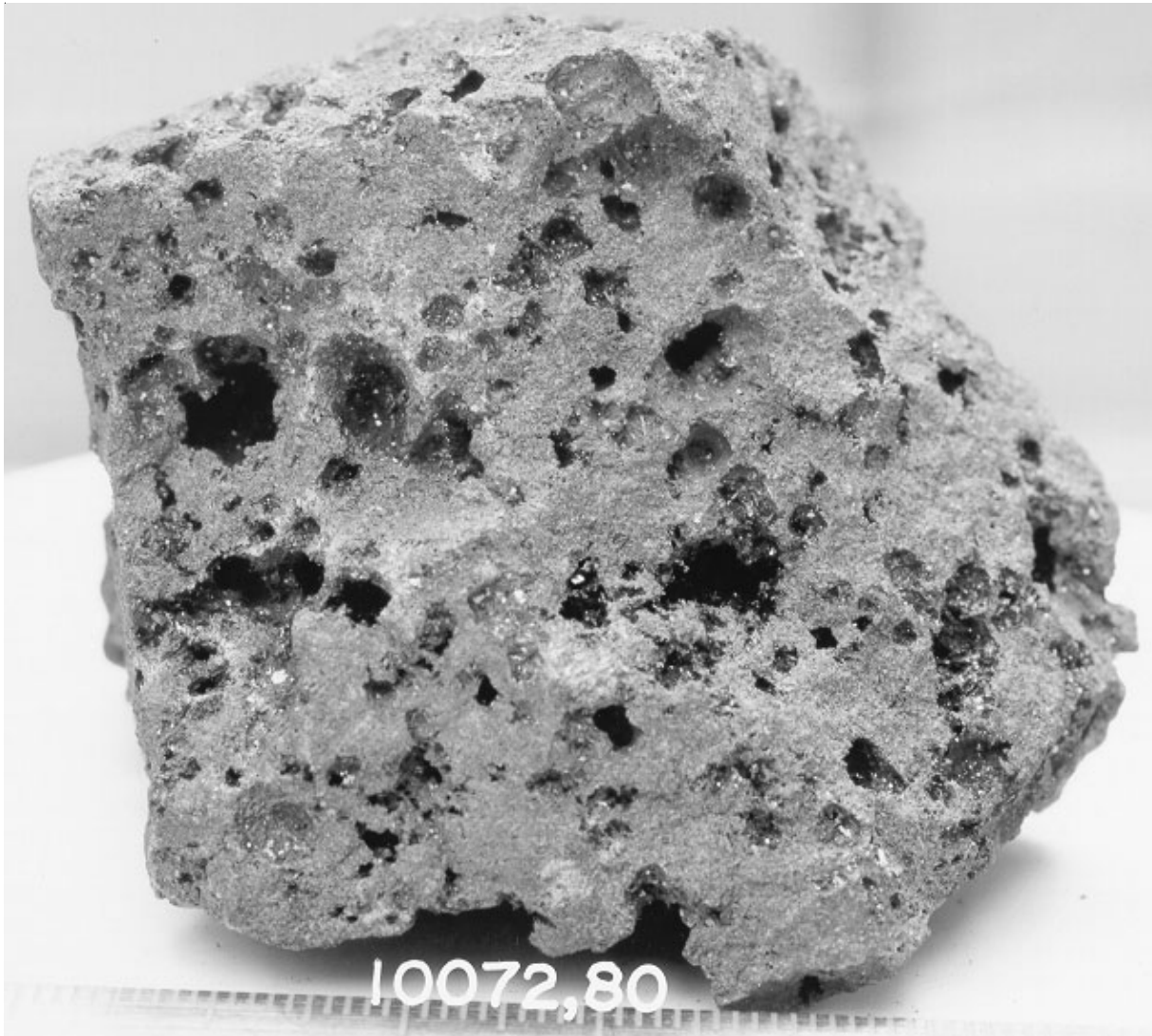
Figure 1: Photo of freshly broken surface of basalt 10072,80 illustrating vesicles and vugs. Sample is about 5 cm across. NASA S76-22599.
