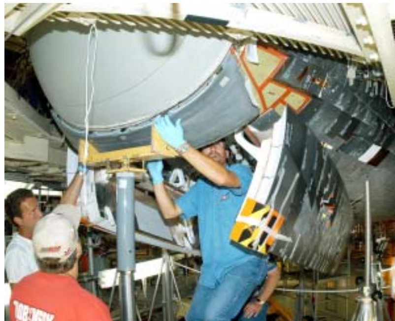
STEPHANIE STILSON, NASA vehicle manager for Discovery, stands under the belly of the orbiter as she explained the advancements made during the spacecraft's ongoing maintenance period. Below, workers in the Orbiter Processing Facility complete the installation of the Reinforced Carbon-Carbon panel on Discovery. The chin panel is the smile-shaped section of RCC directly below the nose cap.
