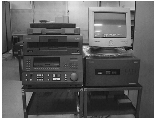
Figure 4. A gigabit VSI recorder.
