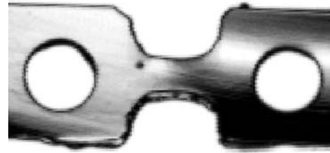
Figure 1: An ultrasound scan of a solder tensile specimen. The image was made by mapping the amplitude of the reflection off the front interface (white = larger amplitude).
