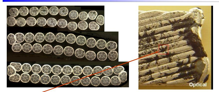
All cables had black spots after reaction at OST. SEM/EDS analysis showed that the black spots included Bi-2212 and MgO. Half a dozen cables were tested at self-fields of 0.1 to 0.3 T. For all, an  $I_c$  degradation of about 50% was measured. The extracted strands were fine and their degradation was less than 20%.
