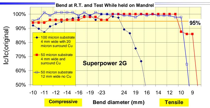
Maximum Bend Strain = +/- t / D ~ 95  $\mu$ m / 11000  $\mu$ m = 0.86 % (~ 0.45 % on the YBCO)
