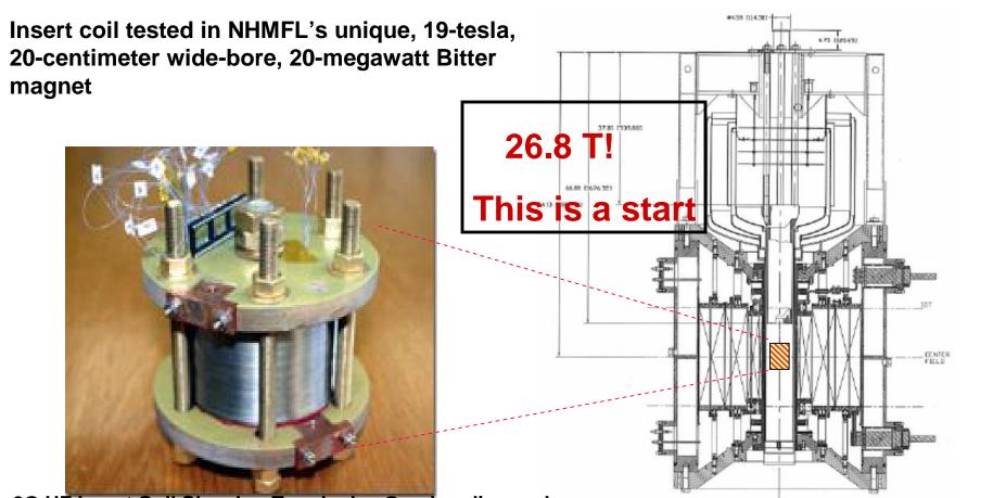
2G HF Insert Coil Showing Terminals, Overbanding and Partial Support Structure. Flange OD is 127 mm.
