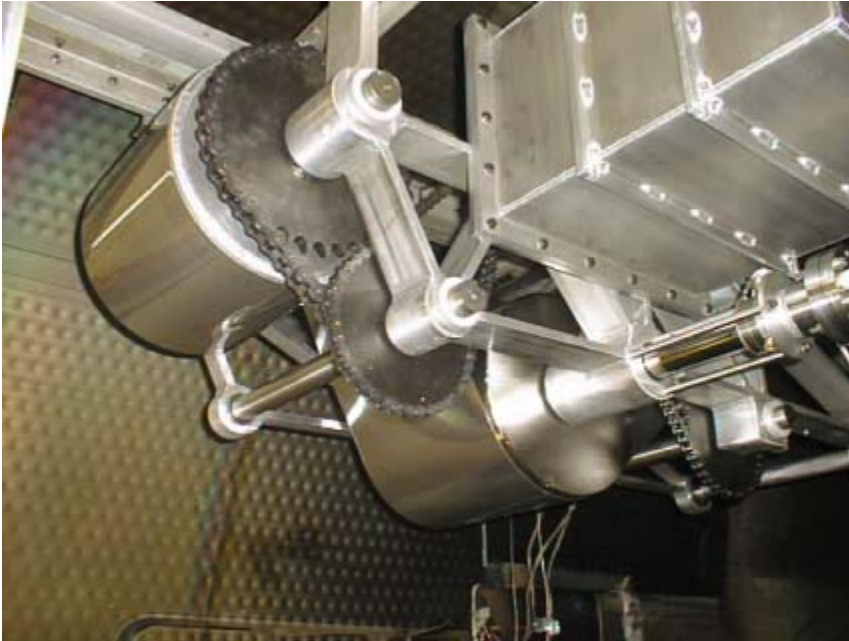
Figure 3b. Backside view of web-handling machine inside the chamber.
