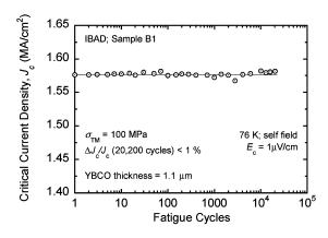
Fig. 3. Dependence of critical-current density  $J_c$  on fatigue cycling under transverse compressive stress up to 100 MPa and 20,200 cycles, in a non-Cu-plated YBCO IBAD slit coated-conductor. The fatigue effect is negligible, showing that propagation of edge cracks induced by conductor slitting is extremely limited.
