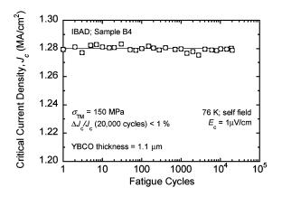
Fig. 4. Dependence of critical-current density  $J_c$  on fatigue cycling under transverse compressive stress up to 150 MPa and 20,000 cycles, in a Cu-plated YBCO IBAD slit coated-conductor. Again, the fatigue effect is negligible, showing that propagation of edge cracks induced by conductor slitting is extremely limited.
