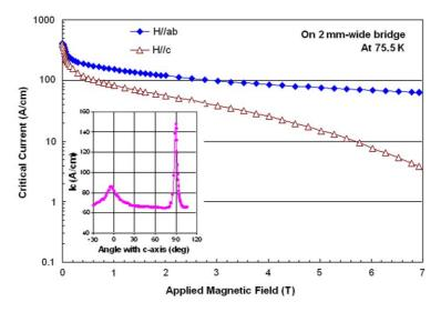
Fig. 6. Field dependence of critical of a Sm-substituted YBCO coated conductor. The insert is the angular dependence of critical current at 1 T.
