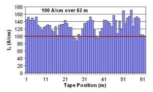
Fig. 5.  $I_c$  profile of a 62 m long MOCVD tape. The end-to-end  $I_c$  is 100 A/cm-width tested by winding the tape on a G-10 mandrel.
