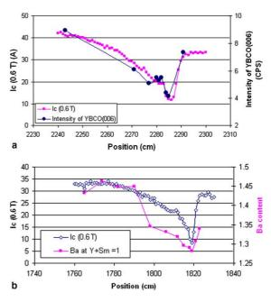
Fig. 3. Data on weak section from the first 50 m run in the prototype MOCVD system.
