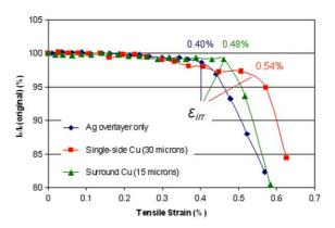
Fig. 8. Normalized  $I_c$  as function of axial tensile strain for three 4 mm wide coated conductors: (a) with only 3  $\mu$ m Ag overlayer; (b) with 30 Cu on YBCO side; (c) with 15  $\mu$ m Cu on all sides.
