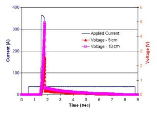
Fig. 7. The voltage response after the 11th 300 ms pulsed current was applied on a 4 mm wide tape with 37  $\mu$ m surround stabilizer. The pulsed current was 364 A, which is 9.1 times of the  $I_c$  of the tape. No substantial degradation in  $I_c$  was observed after this pulse.
