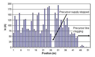
Fig. 2. Critical current ( $I_c$ ) at every meter section of the first 50 m tape processed in the prototype MOCVD system. The voltage criterion is 1  $\mu$ V/cm.
