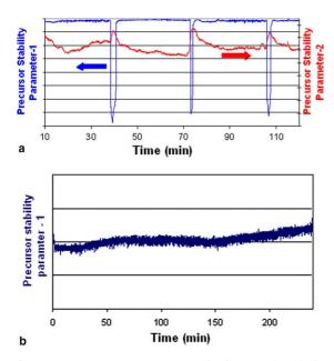
Fig. 4. Precursor parameters monitoring results during MOCVD runs: (a) before system modification; (b) after modifications on the system to solve the precursor parameter instability problem.
