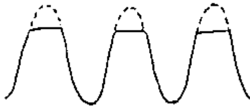
(a) gas supply pressure set too low
