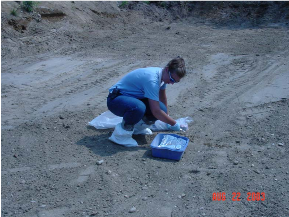
Figure 7: Verification Sampling of Soil Under Ponds
