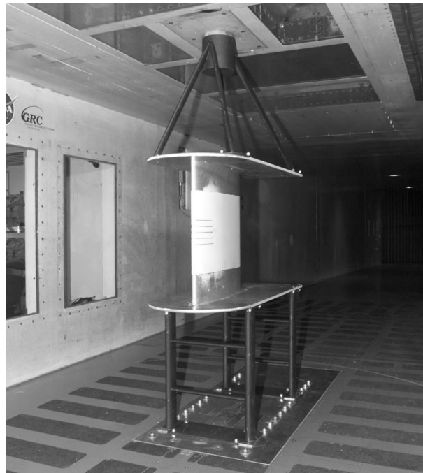
(b) Model Installed in IRT Test Section.
