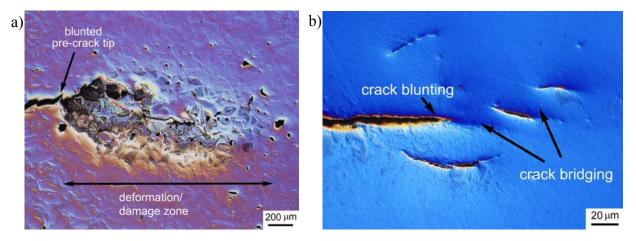
**Figure 3.** Crack blunting seen in alloys (a) C46 and (b) M34 after R-curve testing at 1300°C. Note the order of magnitude difference in scale between the two micrographs.
