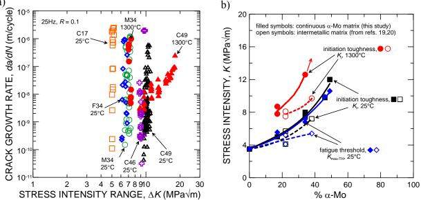
**Figure 4.** Plots showing (a) the fatigue-crack growth behavior for present alloys, and (b) the fracture toughness and fatigue threshold properties of the present  $\alpha$ -Mo matrix alloys compared to that for intermetallic-matrix alloys of similar compositions from refs. [19,20].
