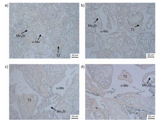
Figure 1. Microstructures of alloys (a) F34, (b) M34, (c) C17, and (d) C46. (C49 is seen in Figure 2b)
