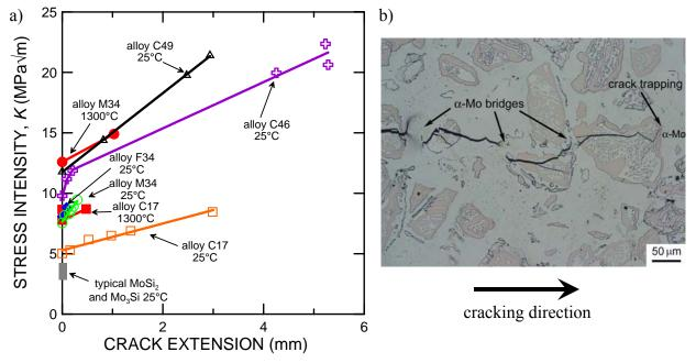
**Figure 2.** (a) shows R-curve behavior for Mo-Si-B alloys, while (b) shows the active toughening mechanisms, crack trapping and bridging by the  $\alpha$ -Mo phase of alloy C49.
