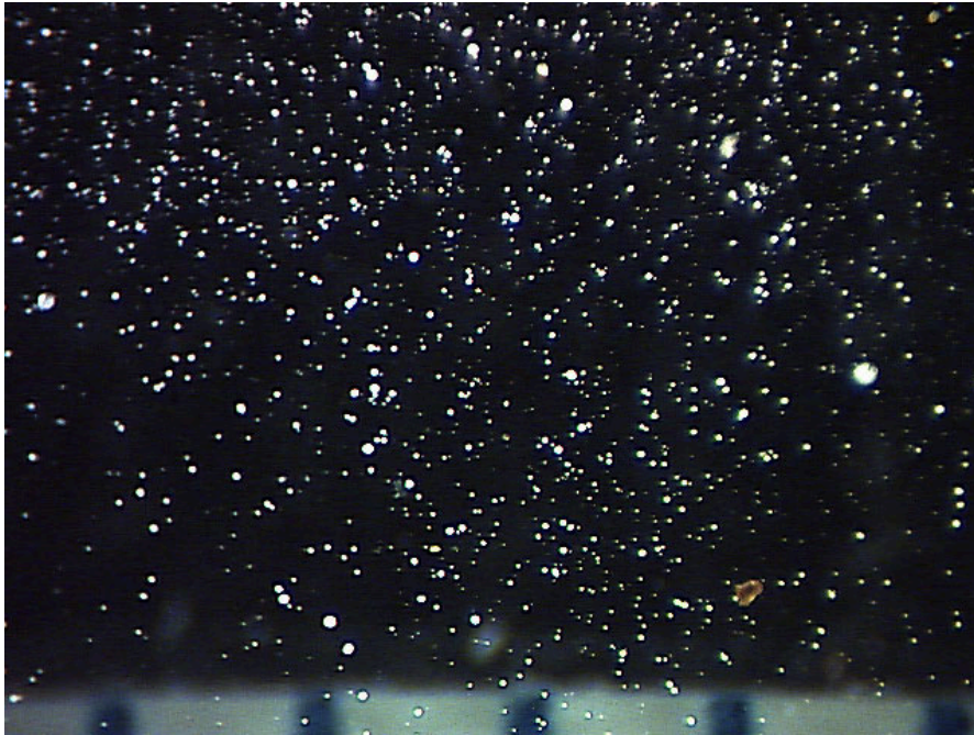
Figure B-17. Large nozzle, test 1f, 2 kg/hr slurry, 3.33 kg/hr atomizing gas, 1,915 NAR.
