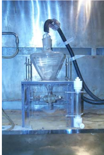
Figure 4. Asbestos sampler glass prototype assembly.
