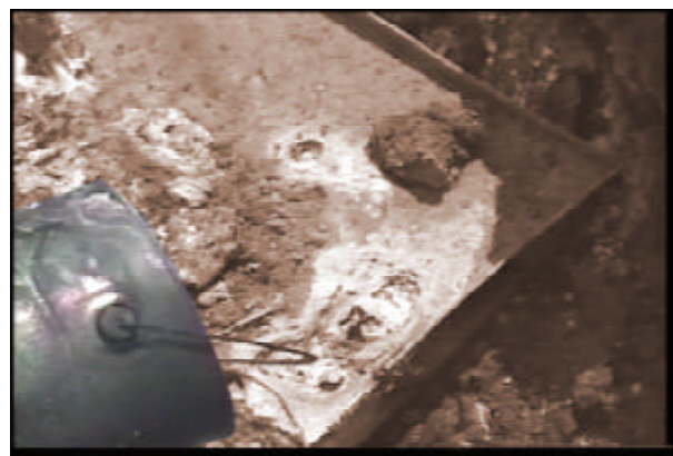
Unburned nitrate residue after cook-off test.
