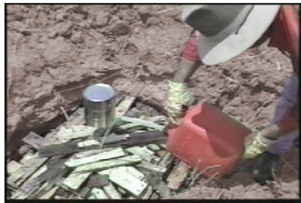
Unburned nitrate residue after cook-off test.
