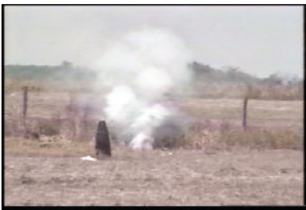
Figure 6-5. White smoke from nitrate burning in cook-off test.
