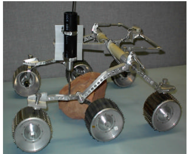
FIGURE 9: Drilling rocks using a USDC that is mounted on a Sojourner class rover.
