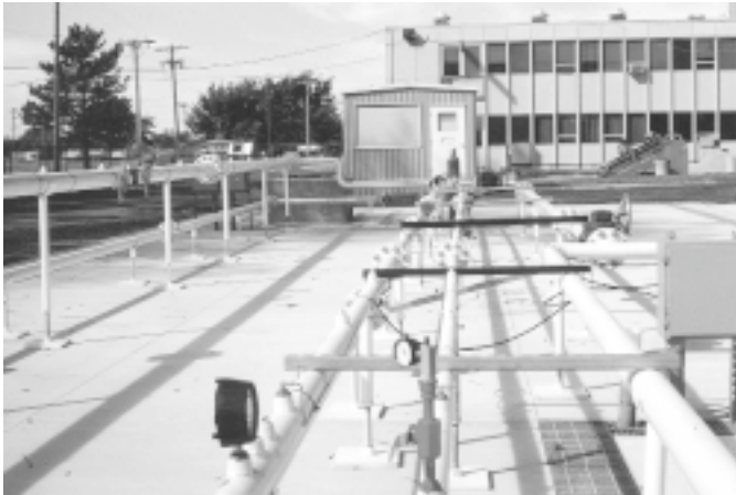
Advanced Cuttings Transport Facility, located at the University of Tulsa, will provide industry with information on the behavior of compressible drilling fluids including foams, which are required to drill and complete wells in depleted onshore and normally pressured offshore oil reservoirs.
