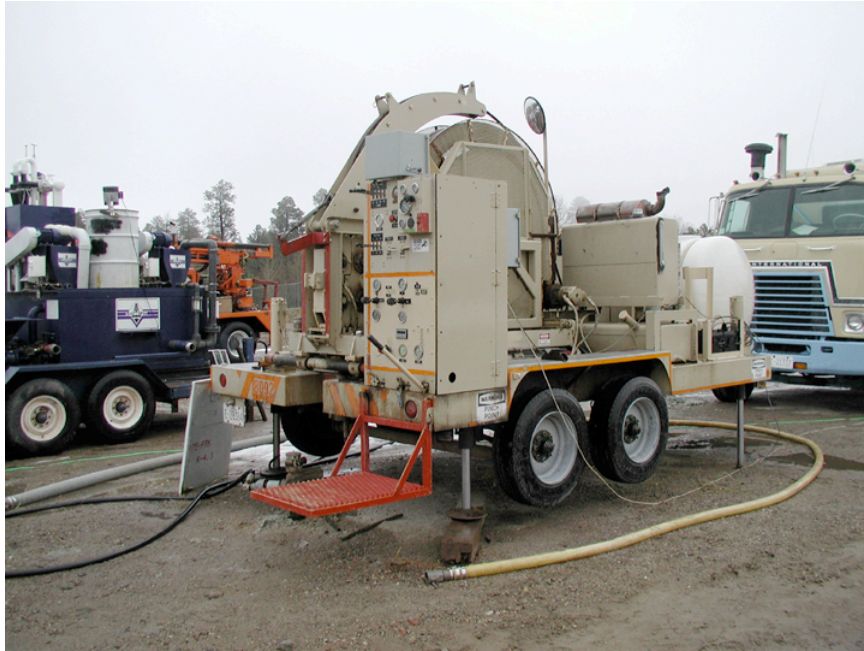
Fig. 8. The Los Alamos coiled-tubing microdrilling rig, (center front), with the mud cleaning system (far left), and the logging van which houses the data acquisition system (far right).
