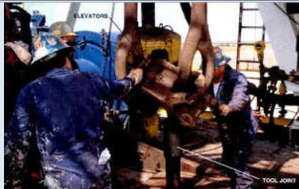
Fig. 5. Elevators latched onto the pipe
