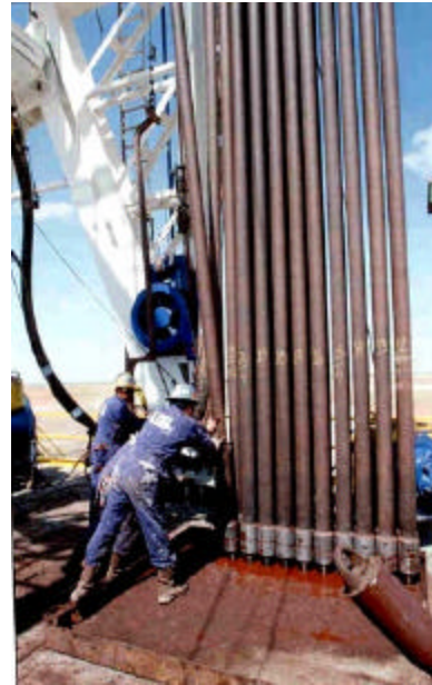
Fig. 1. Setting back a stand of drill pipe
