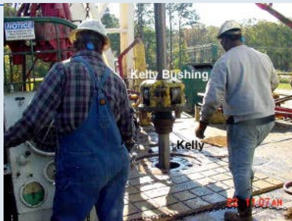
Fig. 15. Lowering kelly bushing
