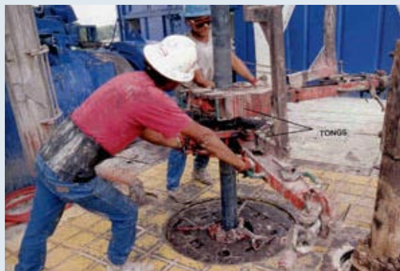
Fig. 9. Using the tongs to breakout the pipe
