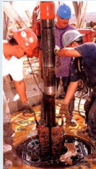
Fig. 8. Setting slips
