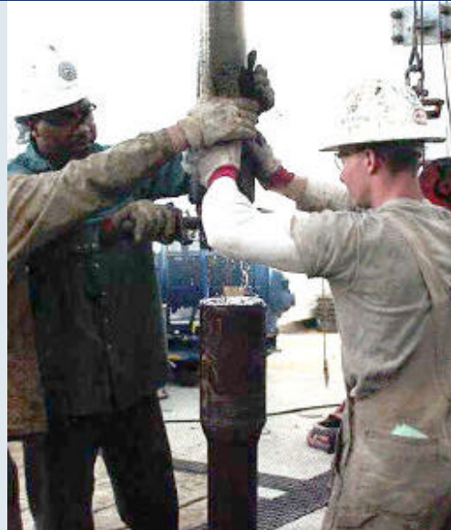
Fig. 13. Applying pipe dope to a connection
