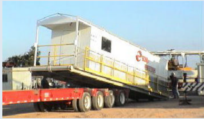
Fig. 19. Loading doghouse onto trailer
