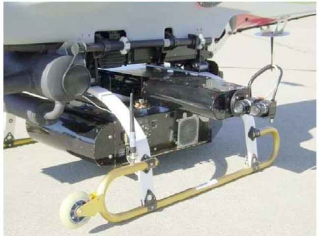
Figure 5. ARP RMAX avionics payload.
