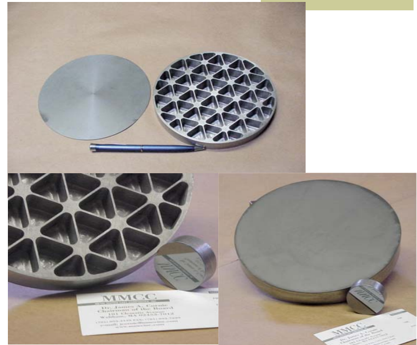
SiC membrane bonded to Mg/Gr lightweight substrate. Part to be Si coated and polished
