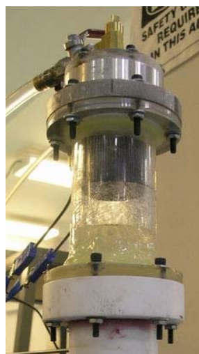
Figure 5. Photograph of third-generation thermosyphon test rig.
