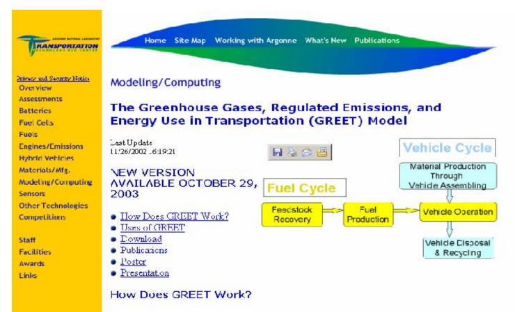
To fully evaluate energy and emission impacts of vehicle technologies, the fuel cycle from wells to wheels and the vehicle cycle through material recovery and vehicle disposal need to be considered. Sponsored by the U.S. Department of Energy's Office of Transportation Technologies, Argorne has developed a fuel-cycle model called GREET (Greenhouse gases, Regulated Emissions, and
